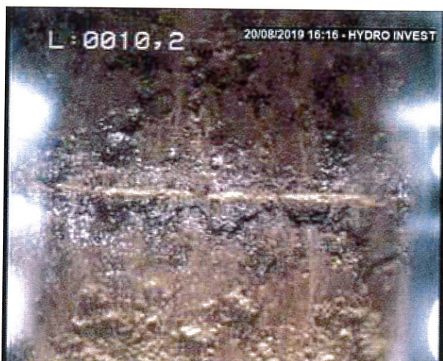
Photo N° 5 – Prof. = 10.2 m/rep Raccord de tube jointif
